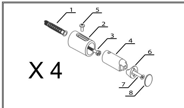
3. There are four sets of wall anchor supports inside the box of accessories.
