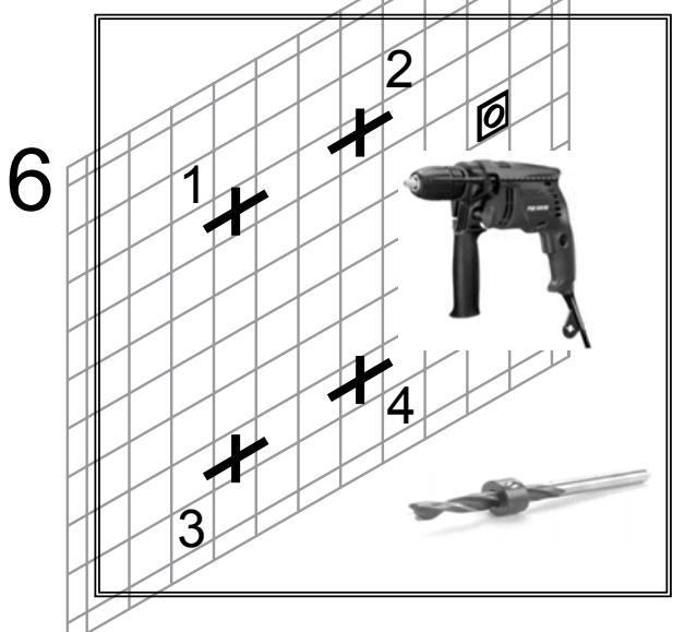
6. Drill the four holes marked on the wall.
