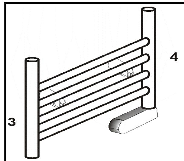
12. Take the HAVERLAND towel-drier radiator and support it on the four supports fixed to the wall. Place the radiator so that the upper supports are between the second and third heater bars.
