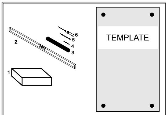
2. Remove the positioning template and box of accessories from the packing box.
