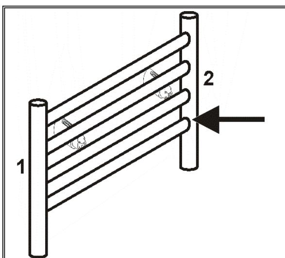
12.- PRENEZ LE RADIATEUR SÈCHE-SERVIETTES HAVERLAND ET APPUYEZ-LE SUR LES 4 SUPPORTS MURAUX FIXÉS AU MUR. PLACEZ LE RADIATEUR DE TELLE SORTE QUE LES SUPPORTS SUPÉRIEURS SOIENT ENTRE LA 2ÈME ET LA 3ÈME BARRE DE CHAUFFAGE.
