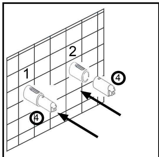
9. Insert the two parts 4 into the upper supports, with the slots upwards.
