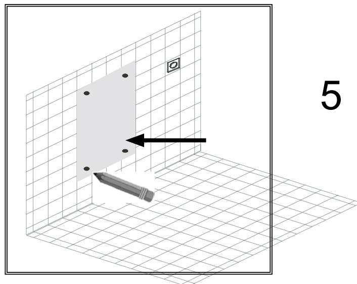
4. Place the positioning template on the wall where the appliance is to be installed and mark the four drill holes.
