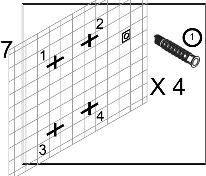
7. Insert the four wall plugs (part 1) into the drilled holes.
