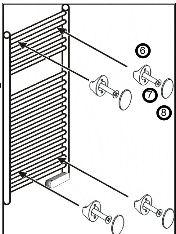
13. Fit the four parts 6 to the wall supports and loosely screw in the four long screws (part 7). Align the towel-drier radiator using a level and, when correctly aligned, tighten the four screws 7.
