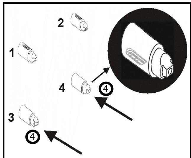
10. Insert the other two parts 4 into the lower supports, with the slots downwards.
