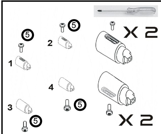
11. LOOSELY screw the four short screws 5 in the four fixing supports.
